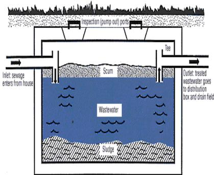
**Tip** To prevent buildup, sludge and floating scum need to be removed through periodic pumping of the septic tank. Regular inspections and pumping are the best and cheapest way to keep your septic system in good working order.
